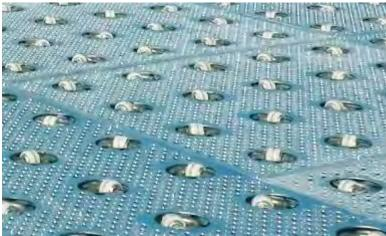
A **toe-guard** prevents operators to step into the holes present in the top deck area while walking over them, pushing the ULD's.
